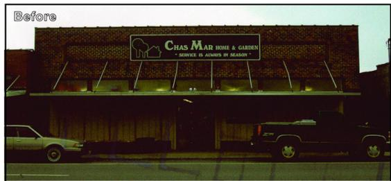
The storefront of the Chas Mar building is in pretty good condition. The brick structure should be inspected, and repaired or repointed if necessary. If cleaning and/or stripping is to be performed, use a gentle water-based or chemical treatment, never sandblasting.
