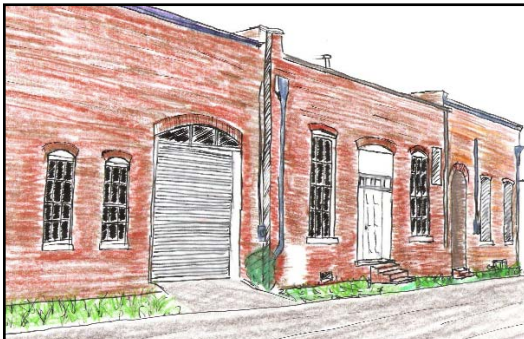
This illustration depicts how the appearance of this building is improved by replacing the windows and removing the HVAC unit.
