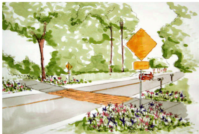
ENSURE SAFE CROSSWALKS WITH RAISED CROSSINGS, CHANGES IN PAVING PATTERNS, AND WELL-MAINTAINED PLANTINGS AT THE INTERSECTION.
