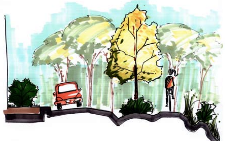
▲ Section illustrating the separation of vehicular traffic from cyclists. The vegetated curbs will assist with stormwater runoff.
