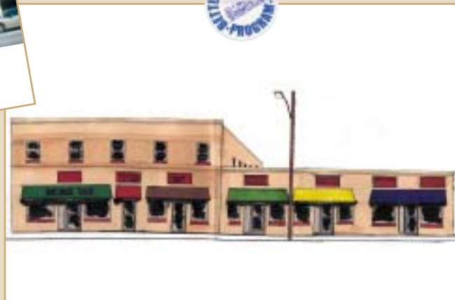
Mansard roofs are removed and traditional awnings added.
