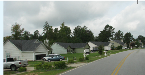
One does not need to go far from the Walnut Grove City Park to find examples of "snout houses." These are buildings designed primarily for the car with the garage occupying a significant portion of the front facade.
