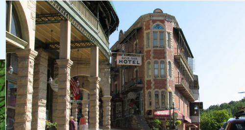
The triangular shaped building at the end of this street is new. The buildings on the left side of the picture are historic. Could you have told the difference? The new building compliments the neighboring buildings through its footprint size, spacing and size of windows, doors and roof shape.
