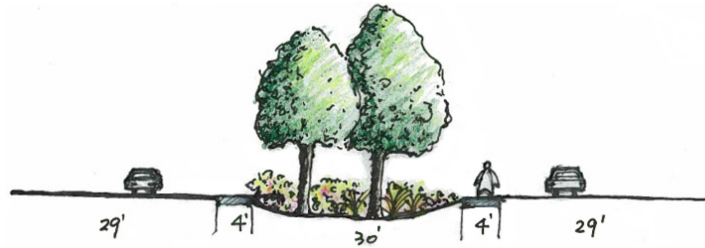
Figure 86 - This section from the student charrette examines how a rain garden would spatially work in the cul-de-sac.
