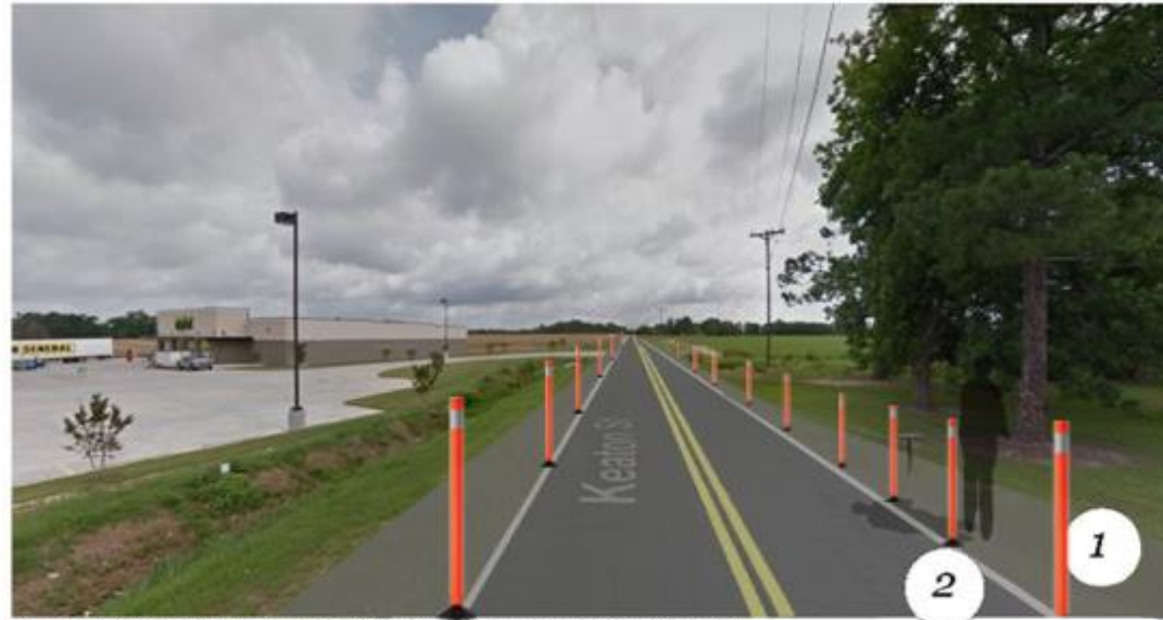
Perspective view of Keaton St. with Advisory Shoulder east of Dollar General Market.
